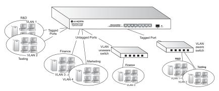
Figure 2-4 Making VLAN Connections
